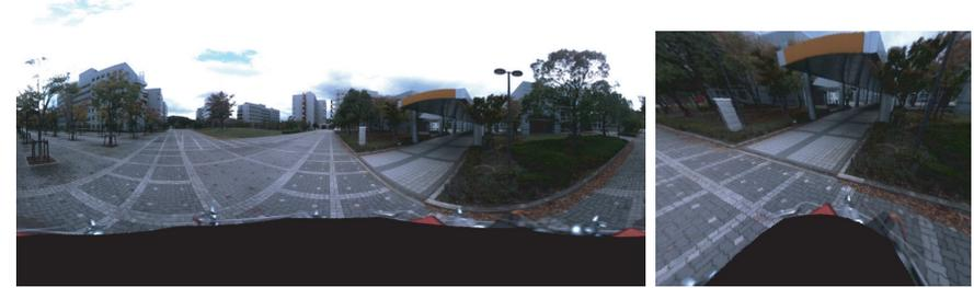
**Fig. 1** Unwrapped spherical panoramic image (left) and a standard perspective image generated from the panoramic image (right). The black regions on these images are caused by the system's inability to capture the area directly below it.
