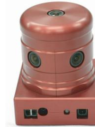
**Fig. 8** Omnidirectional multi-camera system “Ladybug”.
