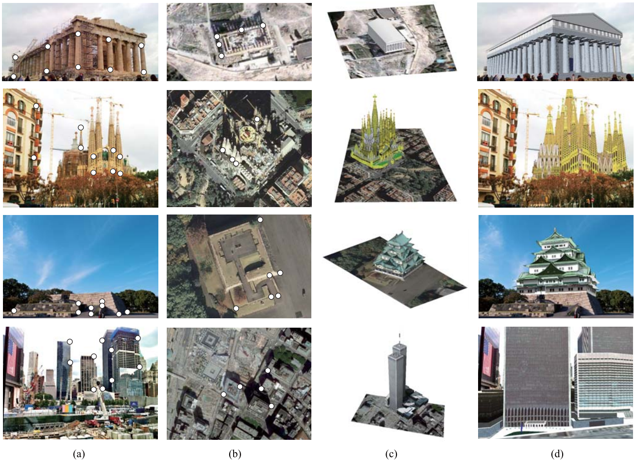
Fig. 13 AR landscape simulations: (a) Internet photographs from Flickr and Google, (b) aerial images from Google Maps, (c) CG objects drawn on aerial images, (d) generated AR images. White points are manually given reference points.
