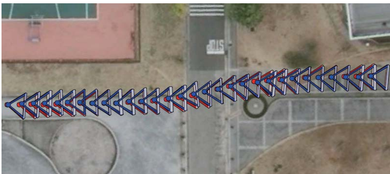
Fig. 10 Camera poses estimated by P5P2D (blue) and ground truth (red).
