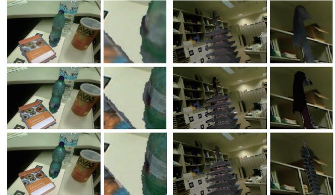
**Figure 7:** Examples of generated AR images. From top to bottom rows: Model-based method, VDT-based method, and proposed method. From left to right columns: generated AR images for DS1 and their close views, and generated AR images for DS2 and their close views.
