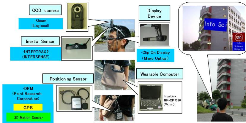
Fig. 4. Hardware configuration of wearable augmented reality system.
