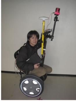
Figure 5 Omnidirectional multi-camera system and GPS receiver.
